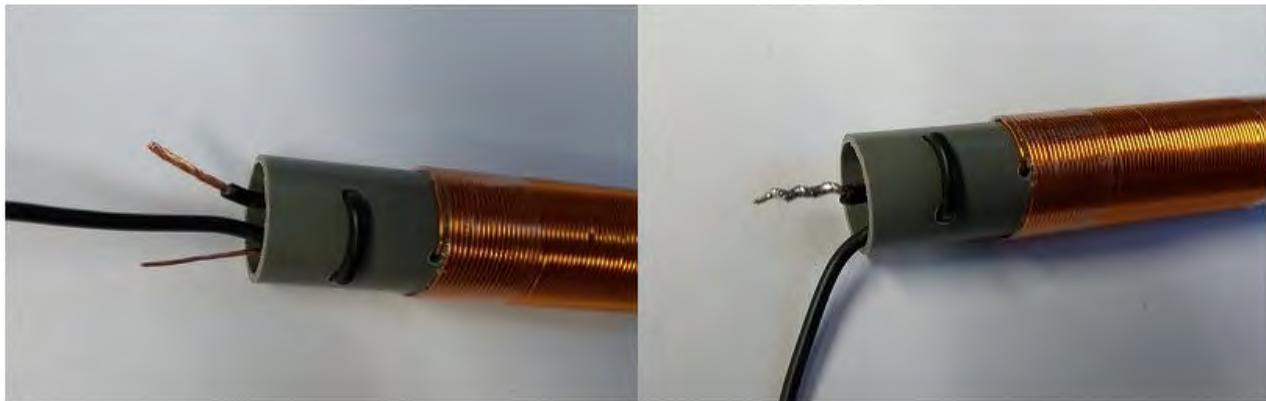
Now cut off the excess winding wire and litz wire to leave just enough length to make a solder. Make sure the winding wire is properly stripped of the enamel layer. This can be done with a sharp knife or sandpaper. Solder the wick to the coil and then insert it into the pipe.
